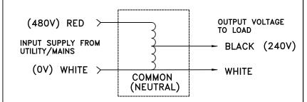
Note: "FB" version has an internal auto reset 110°C thermal protector in series with the "RED" input lead.
